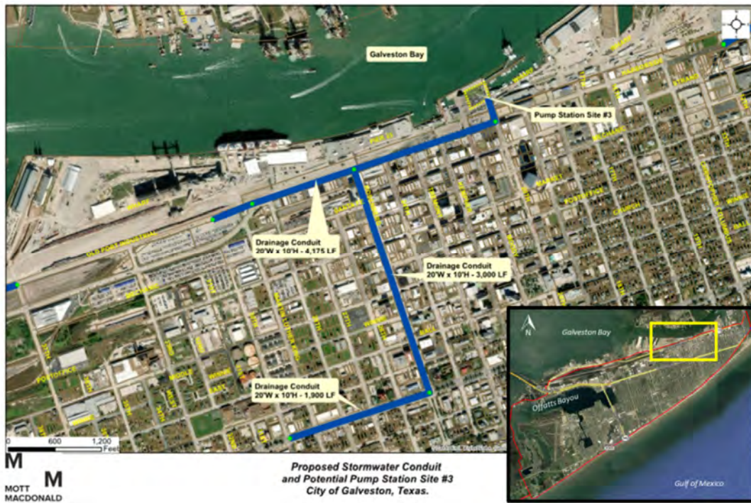
Figure 9. Original proposed stormwater conduit into Pump Site 3.
