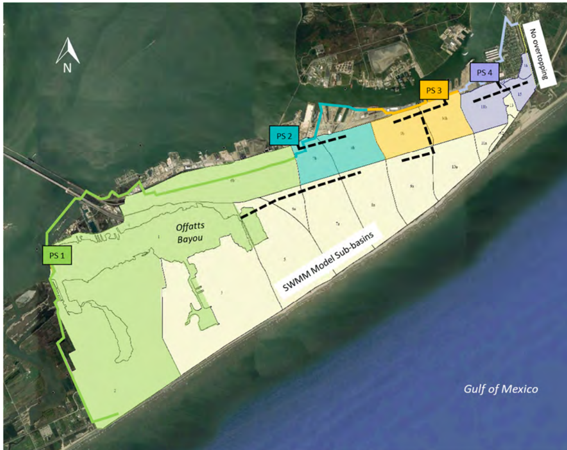
Figure 12. Schematic of the SWMM model sub-basins with the revised alignment. The sections of alignment, sub-basins, and Pump Sites (PS) are color coordinated to show where overtopping contributes to each pump site. No overtopping was observed along the northeastern section of alignment. Note that pump sites and conduit channels (dashed lines) are for visual representations only and do not accurately portray the proposed physical locations of the facilities.
