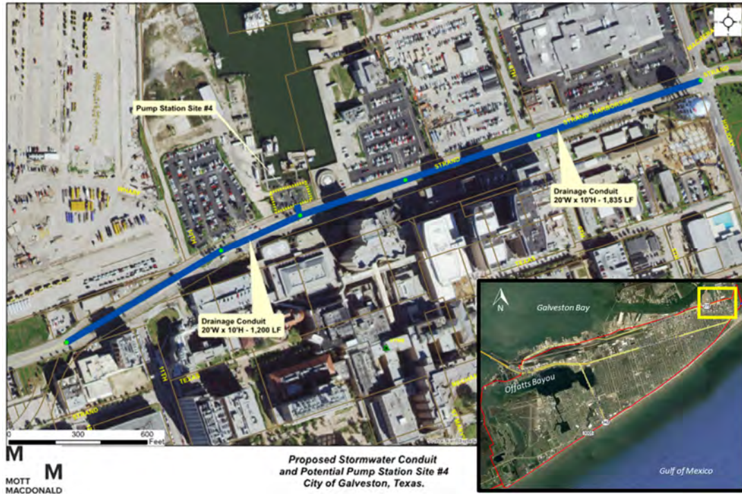
Figure 10. Original proposed stormwater conduit into Pump Site 4.
